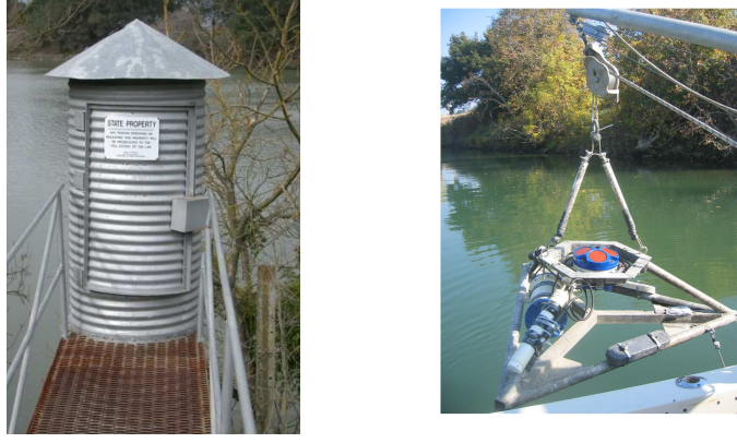
Fig. 7. Left: USGS Sensor station at GSS, used as a measurement sensor. Right: Deployable ADCP sensor, used in Section 3.5 for gathering the validation data (three of them were deployed between 11/01/2007 and 11/12/2007 in order to gather the data for this study).
